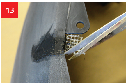
Cut the protruding piece of mesh in the so-called „envelope“...
