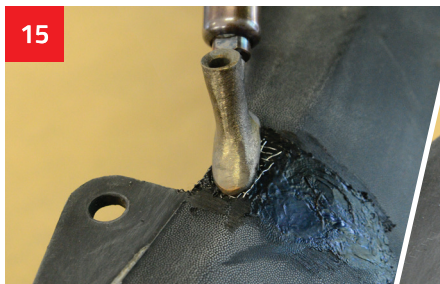
Put the binding material to cover the aluminum mesh completely, and finally even up the repaired area.
