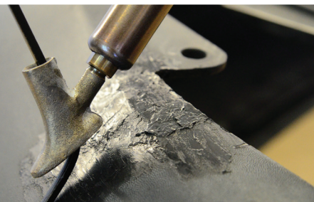
...and fold outwards, setting it in the plastic with the tool.
