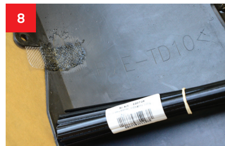
8 To hide the aluminum mesh and strengthen the repaired area, choose the binding material suitable to the type of repaired element.
