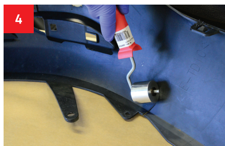
4 Using a roll from the set, smooth the roughness and protrusions.
