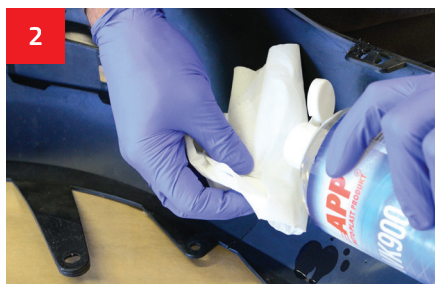
2 Prior to repair, clean and degrease the surface with WK900.
